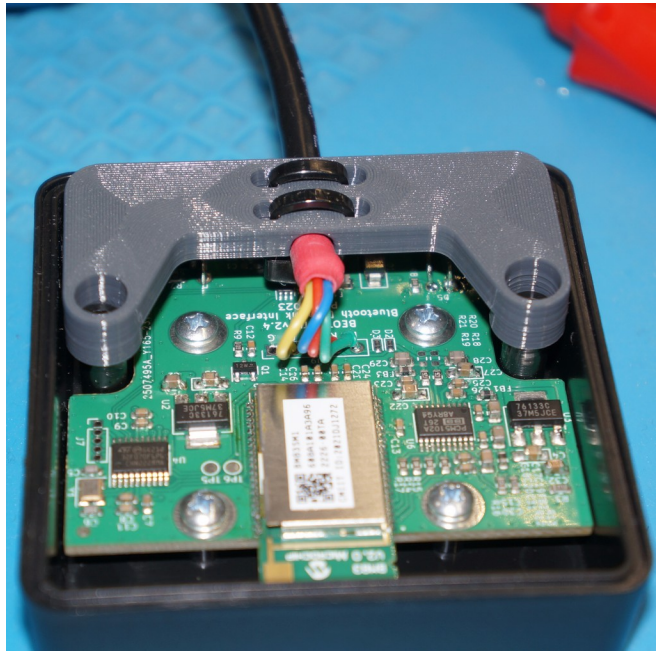
Figure 6: Cable holder in place
