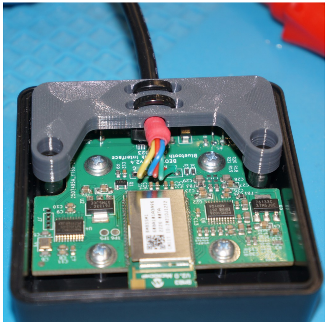
Figure 6: Cable holder in place
