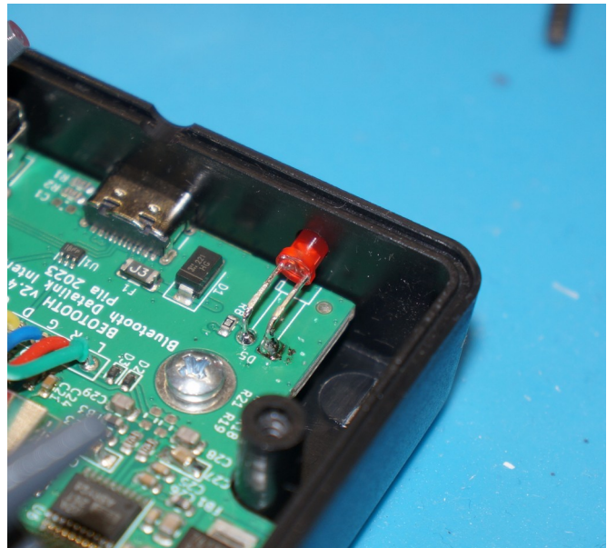
Figure 4: LED soldered to the PCB
