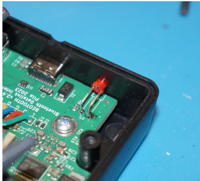
Figure 4: LED soldered to the PCB
