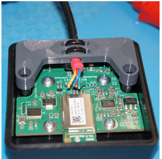
Figure 6: Cable holder in place
