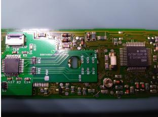
Heat the top of the *GND* pad of the *E-paper interface PCB*, then add some solder so it flows inside the pads. The *E-paper interface PCB* is now mechanically connected to the *upper PCB*, do not attempt to reposition it. If you need to reposition it, make sure to heat the *GND* pad long enough to melt all the solder connecting it to the *upper PCB*.
